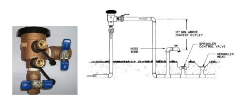
The assembly you need is determined by the hazard. In general, we accept air gaps and reduce pressure backflow assemblies for high hazards and double check valve assemblies, pressure vacuum breaker assemblies and atmospheric vacuum breakers for low hazards.
