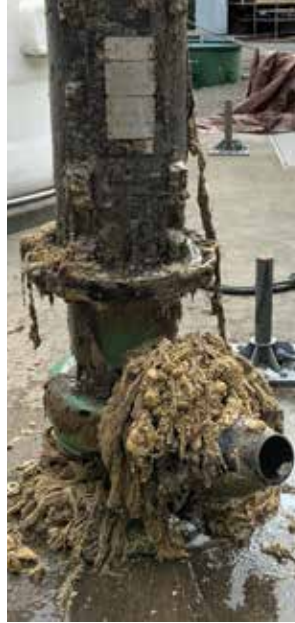
Flushing wipes or other garbage in the toilet increases costs and excess stress on our sewer system, pump stations, and staff.
